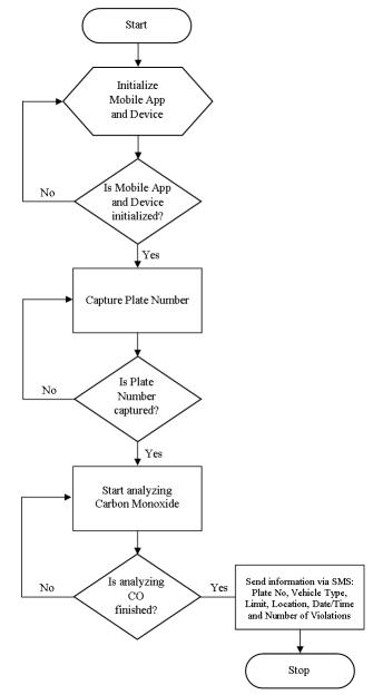
Fig. 3. Flow chart of the vehicle air pollutant monitoring device
