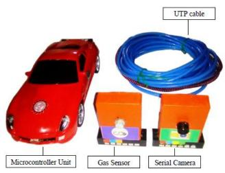
Fig. 2. Vehicle air pollutant monitoring device
