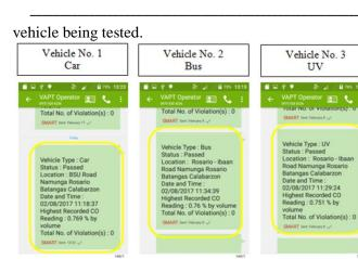
Fig. 5. Sample text messages sent by the vehicle air pollutant monitoring device mobile application
