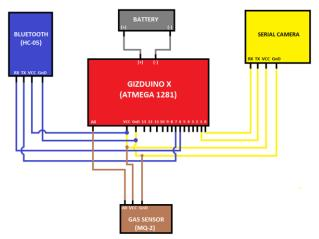
Fig. 1. Schematic diagram of the vehicle air pollutant monitoring device
